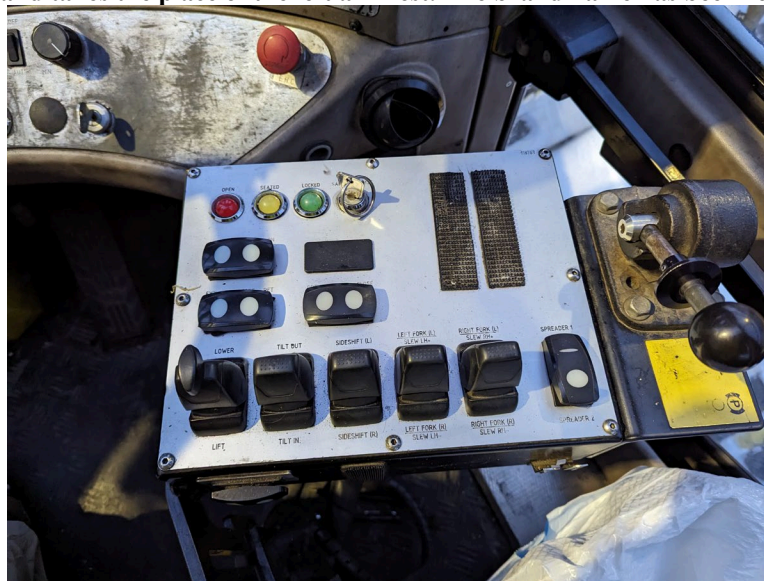
Figure 18. Photo. Mast and pick control panel.
